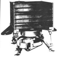
For high screening efficiency plus lightweight sanitary magnesium alloy construction. They provide the ultimate in sanitation, improved product quality, and lower operating costs.
